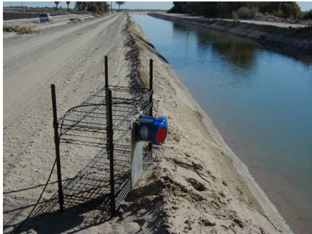
Figure 7 H-ADCP prior to deployment at the California canal site
