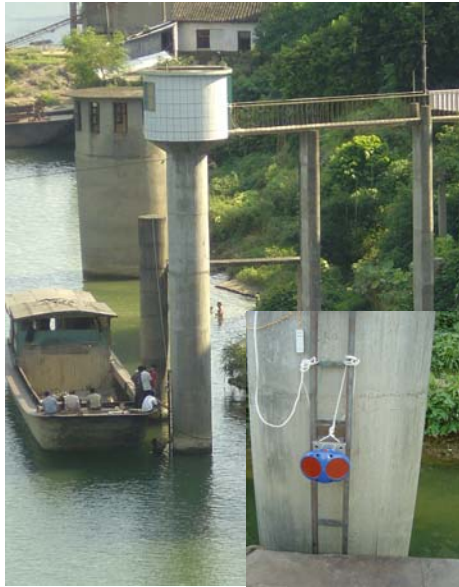
Figure 2 A 600 kHz H-ADCP at Guyi hydrology station in Xiang River, Guangxi, China
