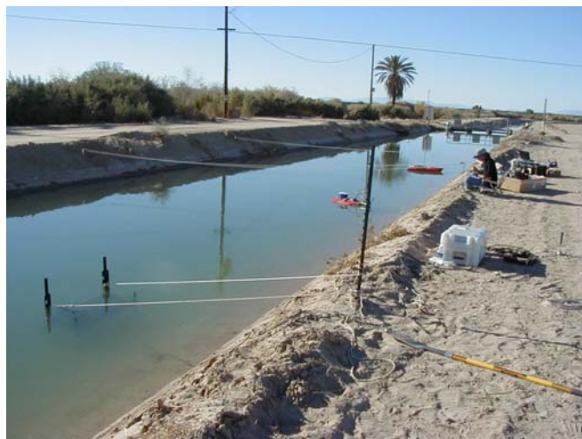
Figure 8 Set-up of H-ADCP and moving-float ADCP at the California canal site
