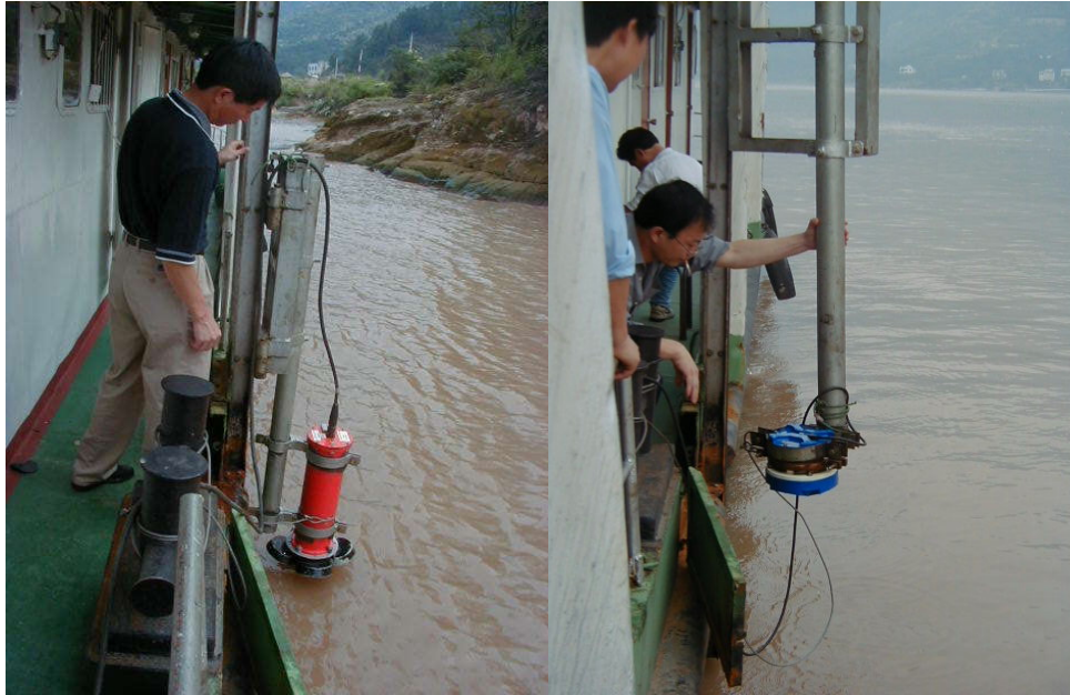
Figure 5 The 300 kHz BBADCP (left) and 300 kHz WHM ADCP (right) mounted on the Huangling Temple hydrology station's survey boat
