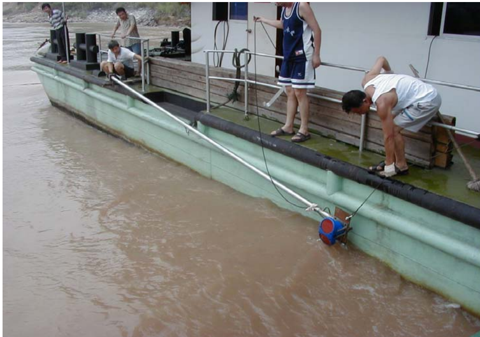
Figure 3 The 300 kHz H-ADCP mounted on the floating dock from March 2004 to March 2006
